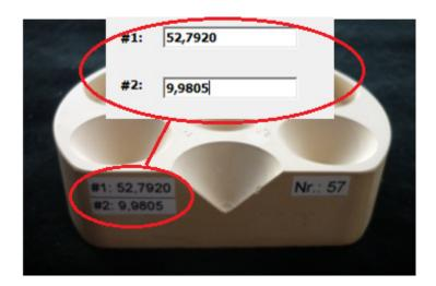
Figure 5: Individual calibration object
