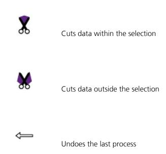
Select a cutting function and click with the left mouse button around the required area. This way you mark the area on and around the model. To conclude the process, perform the last marking with the right mouse button.
