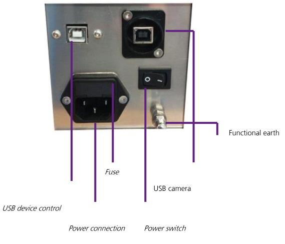
Figure 2: Power switch on the back
