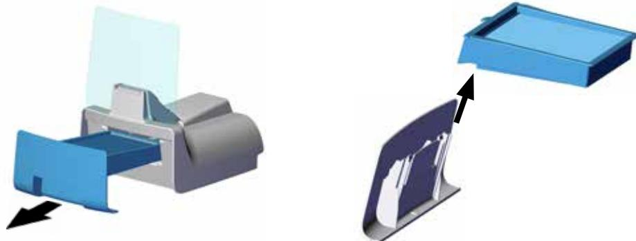
⇒ Remove the dust drawer panel, including the filter element.
